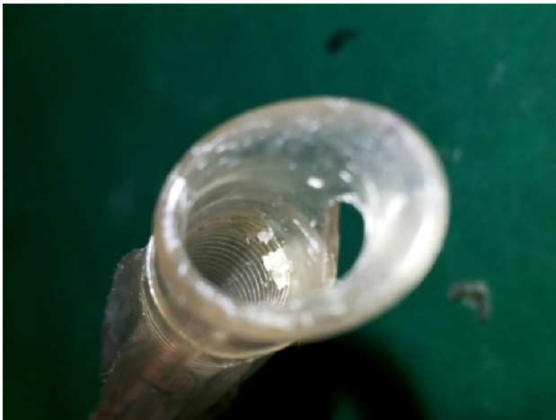
Fig. 2. The same tube after removal of crusts. Note the serrations in the inner wall and retained material corresponding to circular serrations
