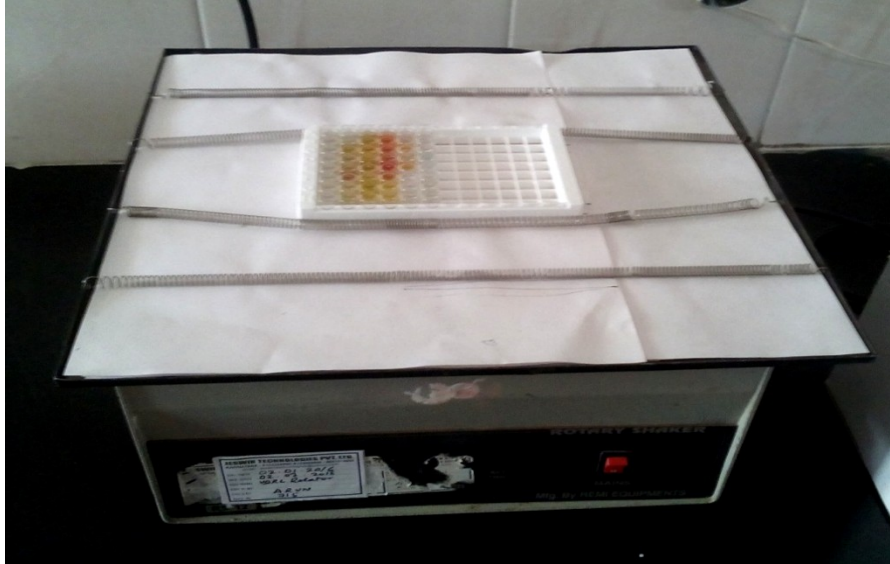
Figure-4.5: Processed EPO microplate incubation on Rotary shaker.
