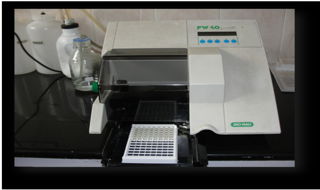
Figure-4.1: Microplate washer (ELISA washer)
