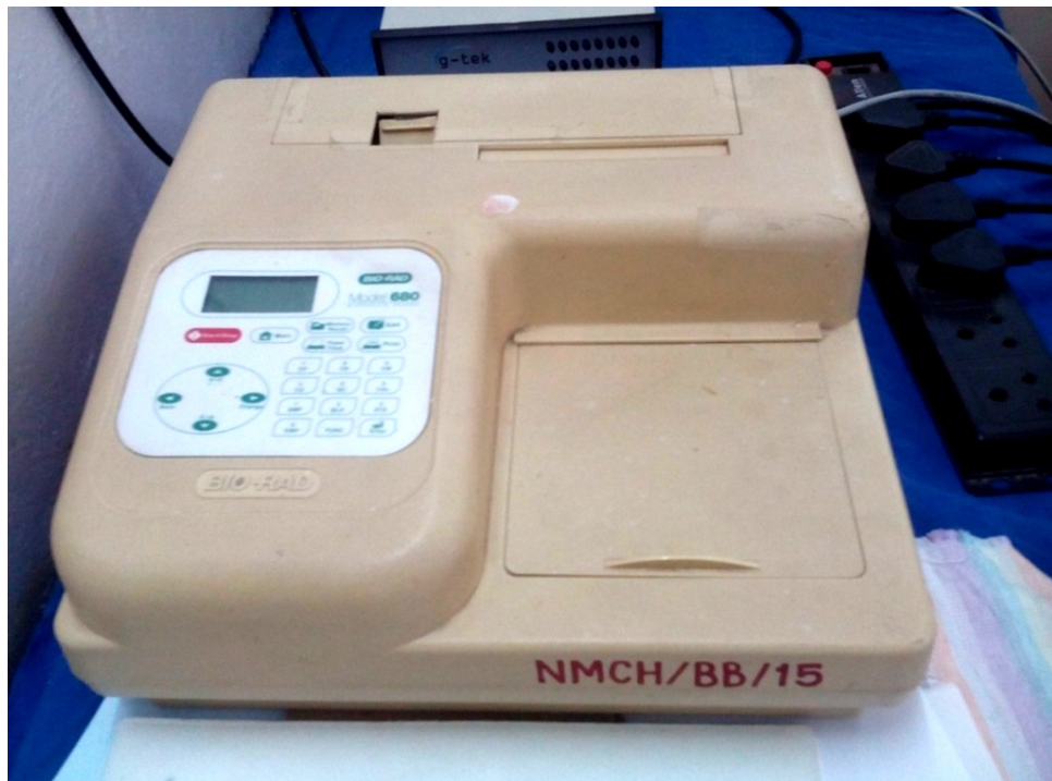
Figure-4.2: Microplate reader (ELISA reader)
