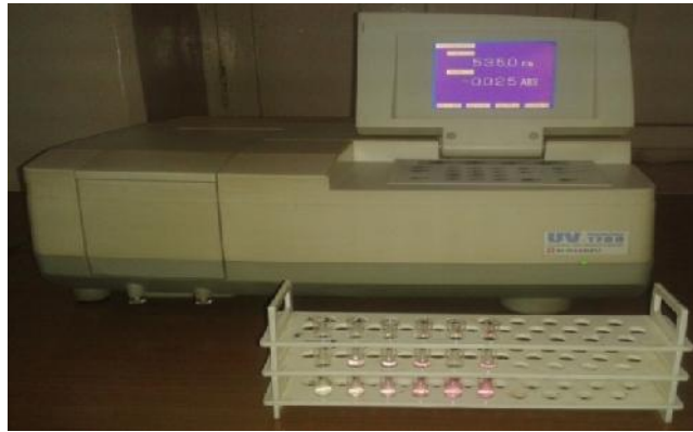
Figure 14: Standard Operating Procedure (SOP) of Melondealdehyde, showing gradual colour change indicate the presence of concentration of Melondialdehyde in S1- S5 test tubes by using Shimadzu UV -VIS Spectrophotometer 1700
