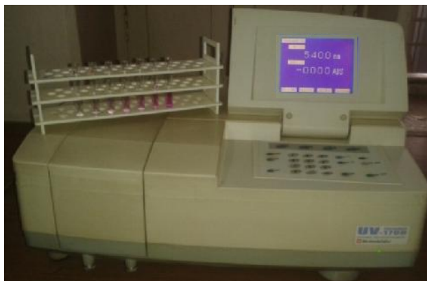
Figure 16: Standard Operating Procedure of Nitric Oxide showing gradual increase in Violet color indicate the presence of concentration of Nitric oxide within the test tubes by using Shimadzu UV -VIS Spectrophotometer 1700
