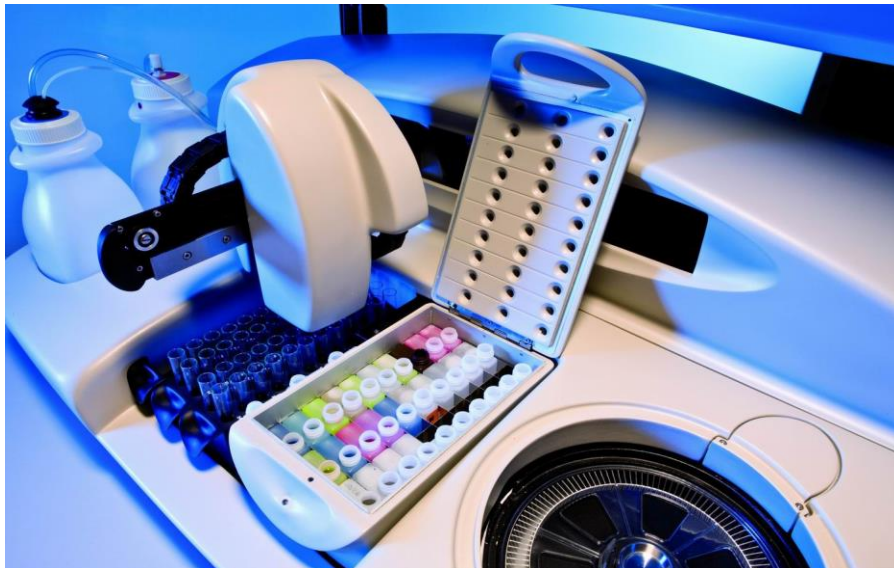
Figure-4.6: Fully automated analyser Biosystem A-25 for biochemical investigations
