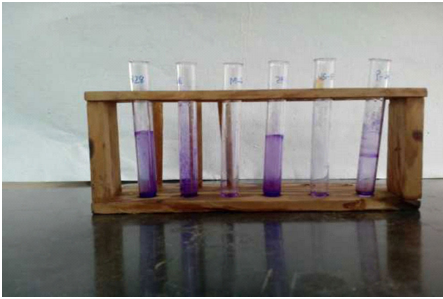
Fig. 1 Biofilm coating the walls of the test tube (violet color)
