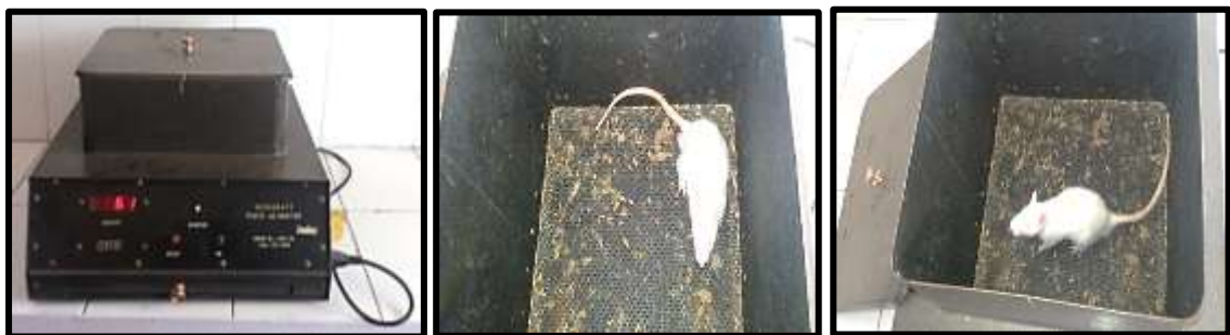
Figure 17: Measurement of locomotor activity using actophotometer [Total number of counts in 10 minutes]
