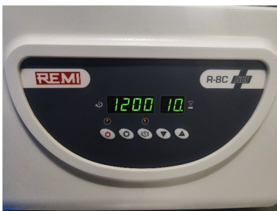
Figure 7 Settings of centrifuge for soft and hard spin.
