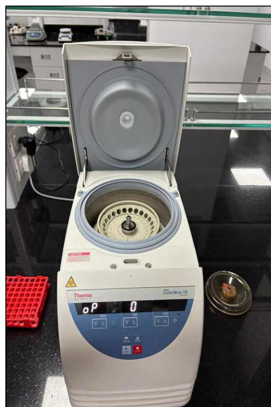
Fig 15: Tabletop centrifuge machines used to centrifuge serum
