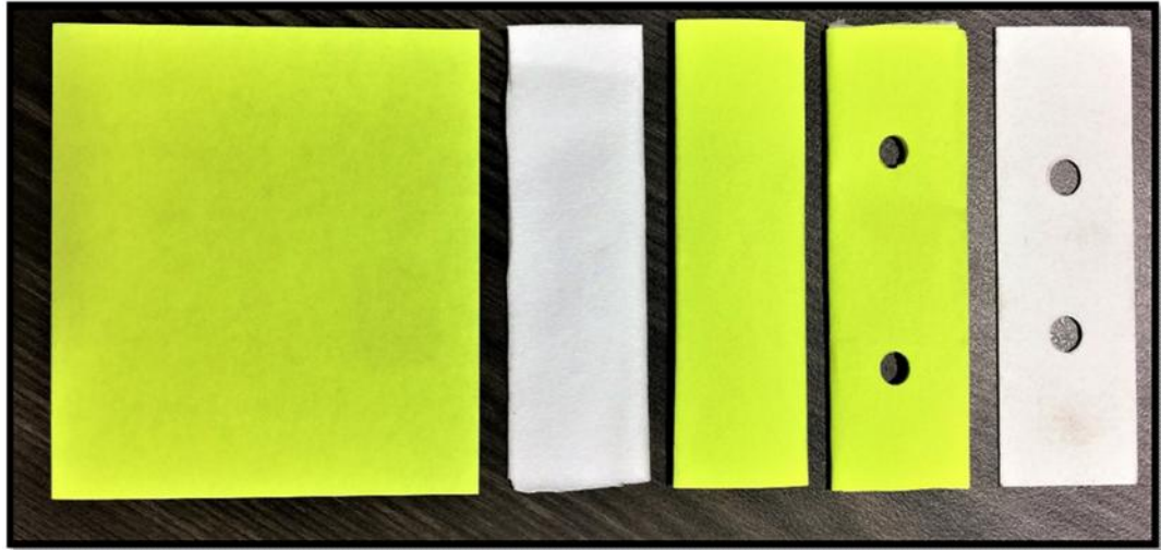
Figure 41 Steps of Preparation of Post it and tissue paper cytofiltration card, extreme right Manufacturer provided Cytofiltration card for comparison.
