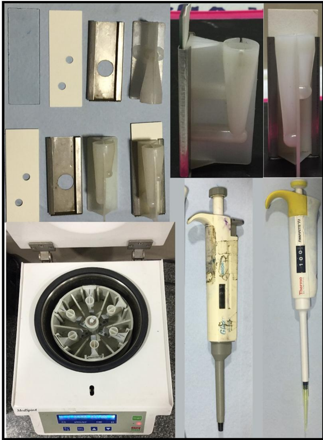
Figure 5 Assembled Cytofunnel, Pipettes and cytofunnels in the cytocentrifuge ready for processing.
