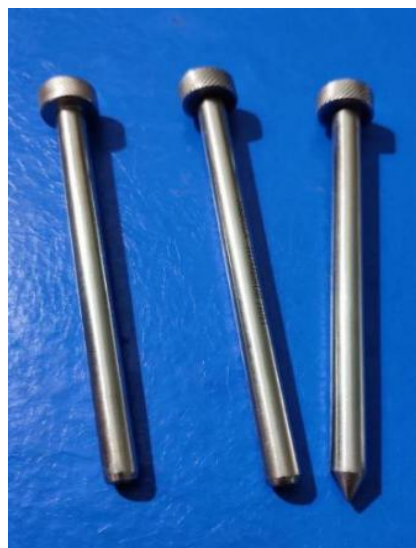
Fig 15.3 : Protection sleeve and trocar
