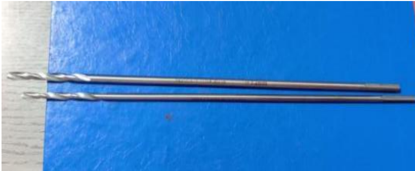
Fig 15.8 : Drill bit 3.2mm and 2.2mm
