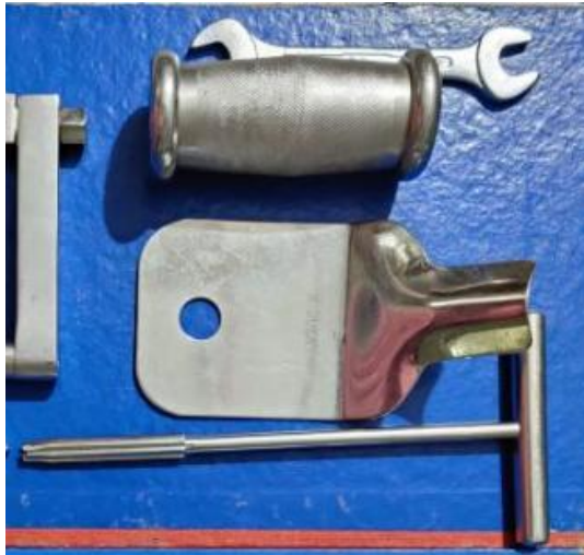
Fig 15.4 : entry reamer and ram
