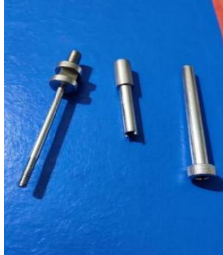
Fig 15.7 : Conical bolt/ Insertion bolt
